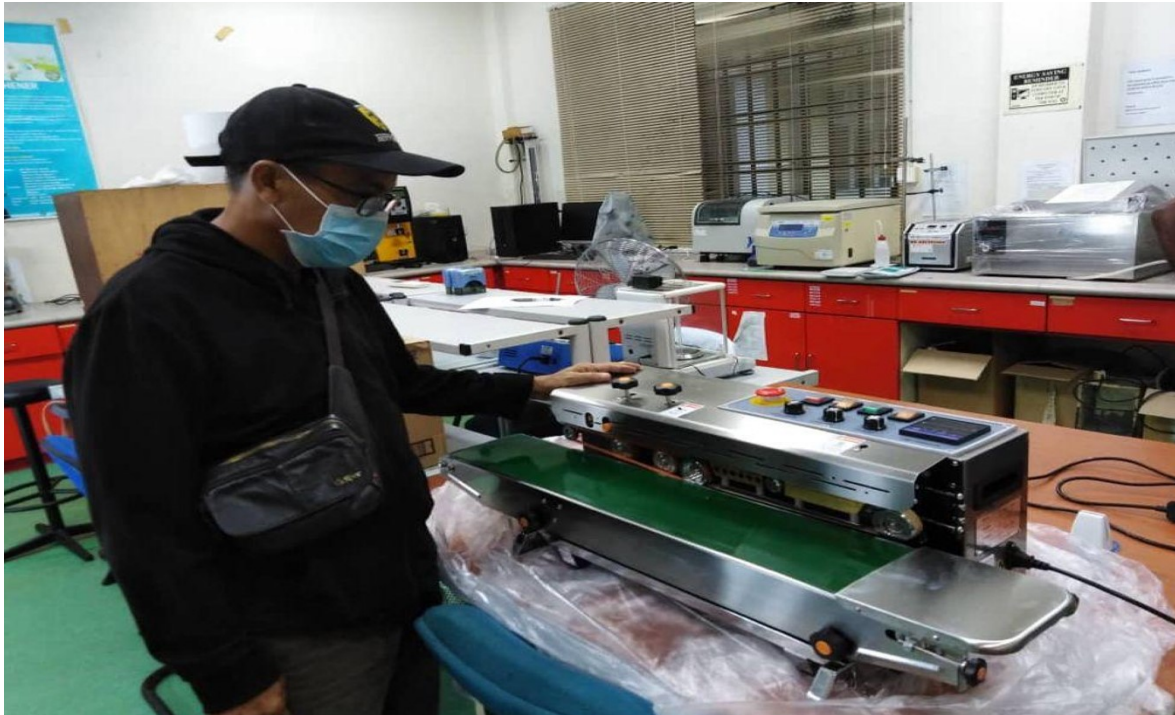
Figure 2 A Lab Assistant testing the Continuous Sealing Machine at UTM FOODI Lab before students using it for their Food Packaging course of MSc FOODI
